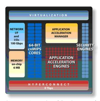
The SSBC i720 takes full advantage of the revolutionary new application acceleration engines. OCTEON II IAP's scale from 1 to 32 cores, including up to 75 Application Acceleration Engines, providing an aggregate performance of over 120 billion operations/second.
